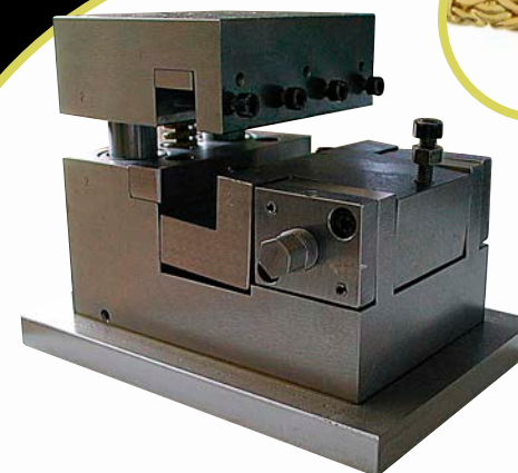
ATTREZZO A CONTENERE PER BATTERE CATENE (100mm) SPECIAL EQUIPMENT FOR HAMMERING CHAINS (100mm)
